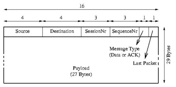
Figure 6: Transport protocol packet
