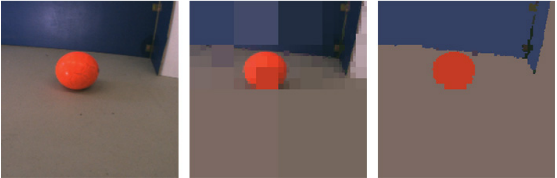
(a) original 256 \times 256 24-bit picture, (b) result after Merge: 748 regions, (c) result after Grouping: 19 regions.
