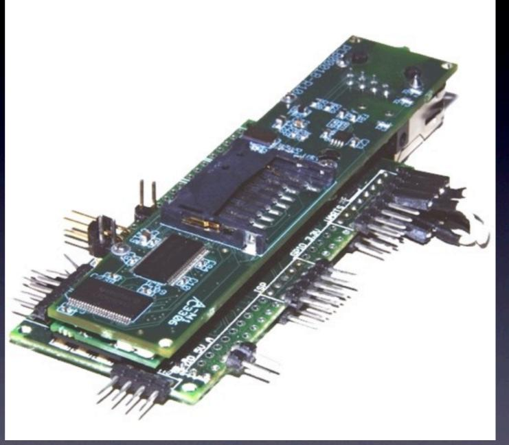
600MHz XScale, I28MB RAM, WLAN, Atmega uController
