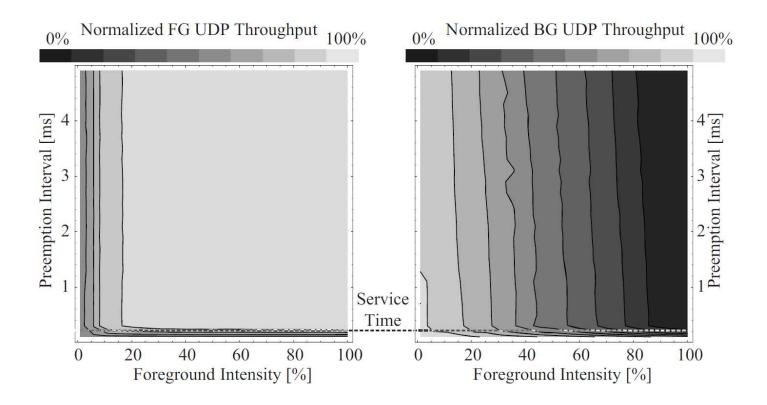
1 Gbit/s interface, UDP transmission to discard service (1400 Bytes/packet) Service time 0.05 ms (measured), orders of magnitudes less than inter-arrival time for foreground requests (100 ms)
