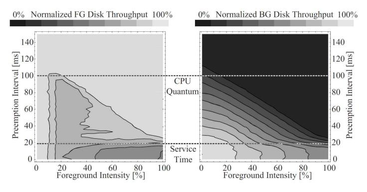
Random access on 8.2GB ATA disk: seek time (15ms) + mean latency (5ms) = service time (20ms) Reading 512 byte blocks
