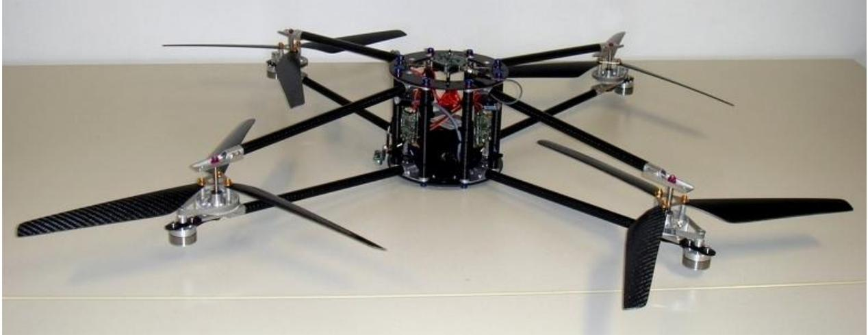
**Figure 3.** The JAviator: a custom-built quad-rotor helicopter used for experiments in this paper ([javiator.cs.uni-salzburg.at](http://javiator.cs.uni-salzburg.at))
